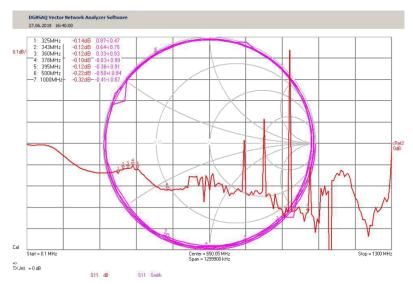
The figure on the left shows an S11 measurement from 0.1 MHz to 1300 MHz with 201 measurement points and maximum measurement duration (VNWA Settings Sweep) after calibration with the Magi-Cal. More spurious responses are visible at frequencies above 500 MHz and at the highest frquencies the VNWA becomes slightly less accurate, but it still shows a very acceptable calibration of the VNWA.
